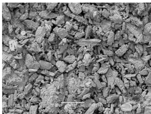
Figure 8. Representative microstructure of a TDF (2.5% maltitol at 55% saturation level) observed with a scanning electron microscope.
